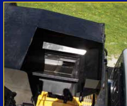
The 50/50 split hopper includes a hydraulic crusher panel that keeps refuse and recyclables or two types of trash separated.
