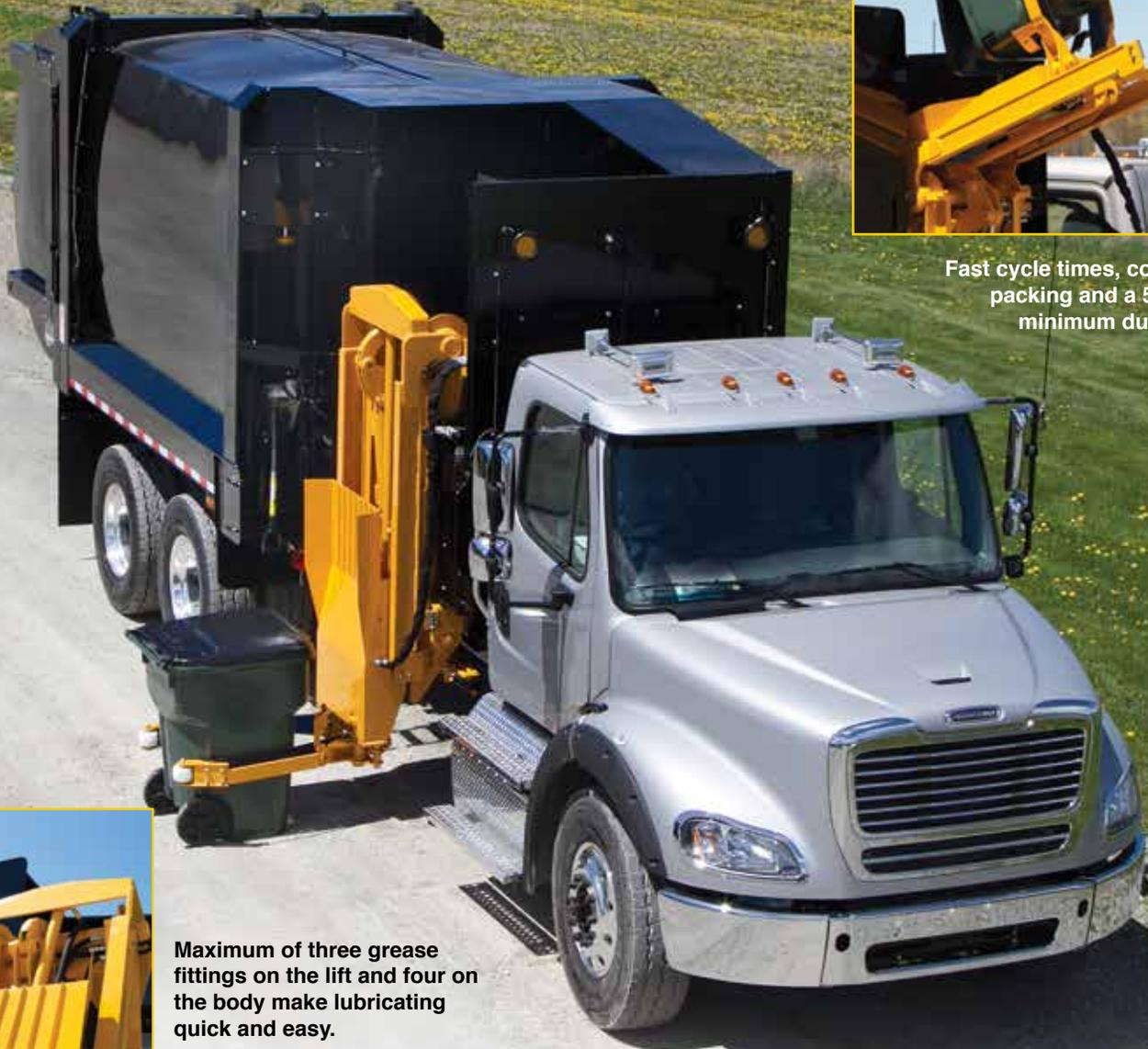
Maximum of three grease fittings on the lift and four on the body make lubricating quick and easy.
