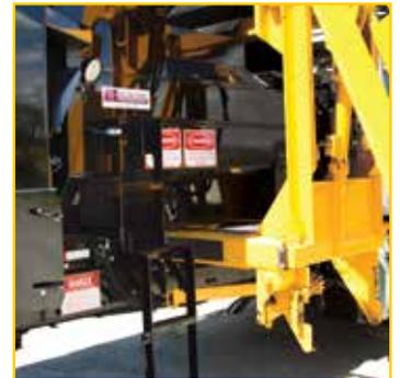
Folding ladder allows for safe and easy access to the hopper.
