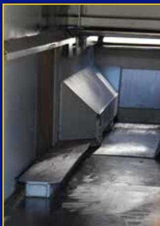
Safe horizontal ram eject unloading eliminates costly multi-stage cylinders. Hardox® wear plates and secondary reinforced welds makes the CS9200SB one of the toughest split bodies on the market.
