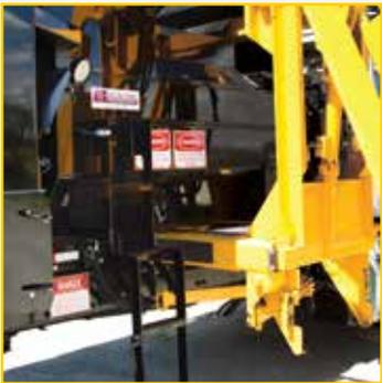
Folding ladder allows for safe and easy access to the hopper.
