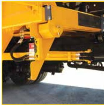
Hydraulic lines are neatly contained and tucked away during arm retraction.
