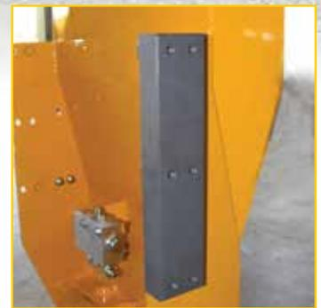
Featuring Nylatron® non-lube wear guides—horizontal slide guides are replaceable without track disassembly.
