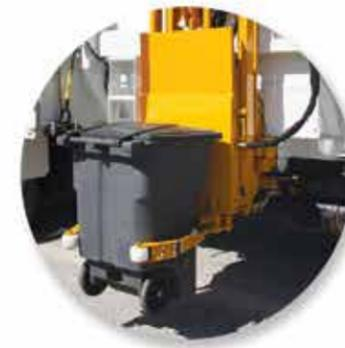
A 38" straight vertical lift before the cart tips allows for easy collection off of retaining walls and snow banks.
