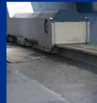
Hardox® wear plates and secondary reinforced welds
